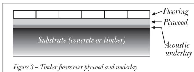
Figure 3 – Timber floors over plywood and underlay
