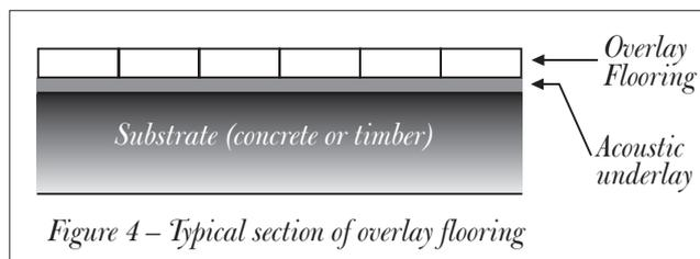
Figure 4 – Typical section of overlay flooring
