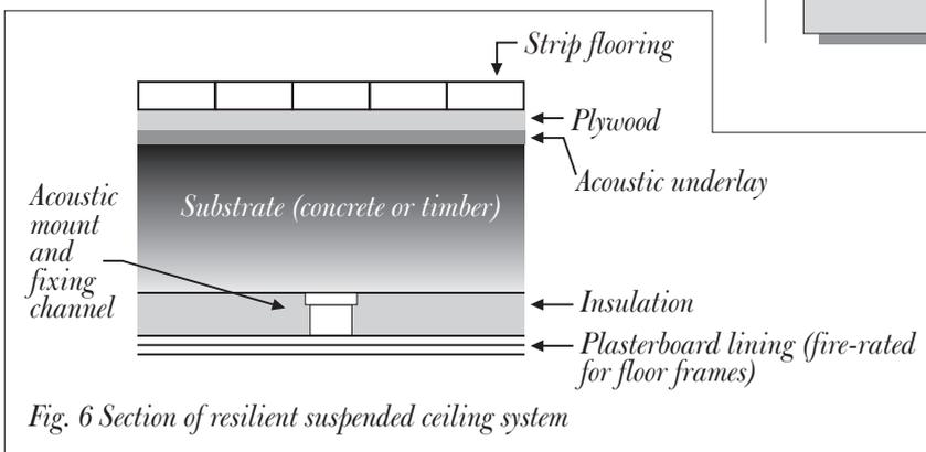
Fig. 6 Section of resilient suspended ceiling system
