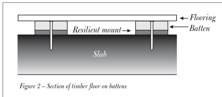
Figure 2 – Section of timber floor on battens
